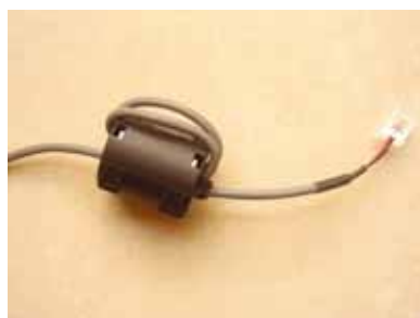
Connection Manner of Crystal Connector, Communication Line and Magnetic Ring
