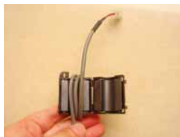
Connection Manner of Crystal Connector, Communication Line and Magnetic Ring
